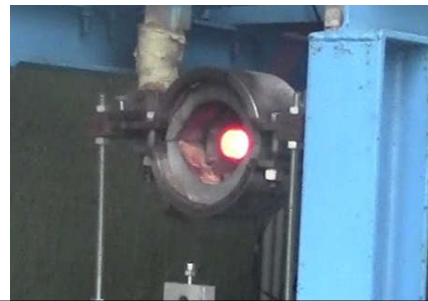
Hybrid rocket exhaust nozzle after the engine burn-out for Test HDPE-1
